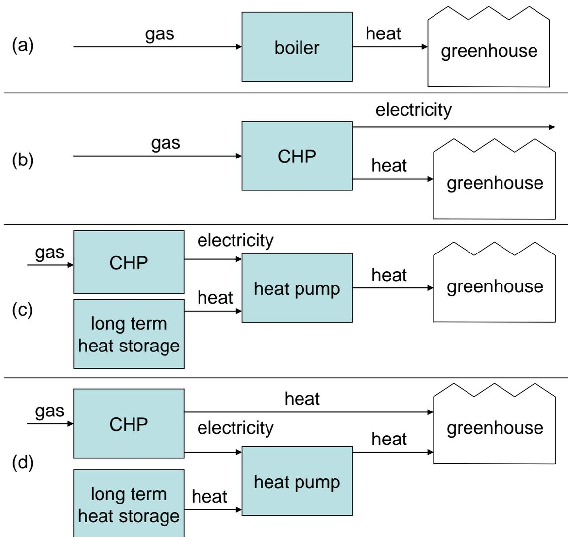
*Fig. 1. Schematic representation of the energy supply systems: (a): the conventional system consisting of a boiler in combination with a condenser; (b) the combined heat and power installation cogeneration; (c) the electric driven heat pump; (d) the gas powered heat pump*
