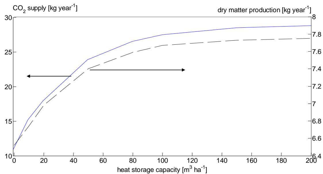
Fig. 2. The carbon dioxide supply and dry matter production as a function of the short term heat storage capacity
