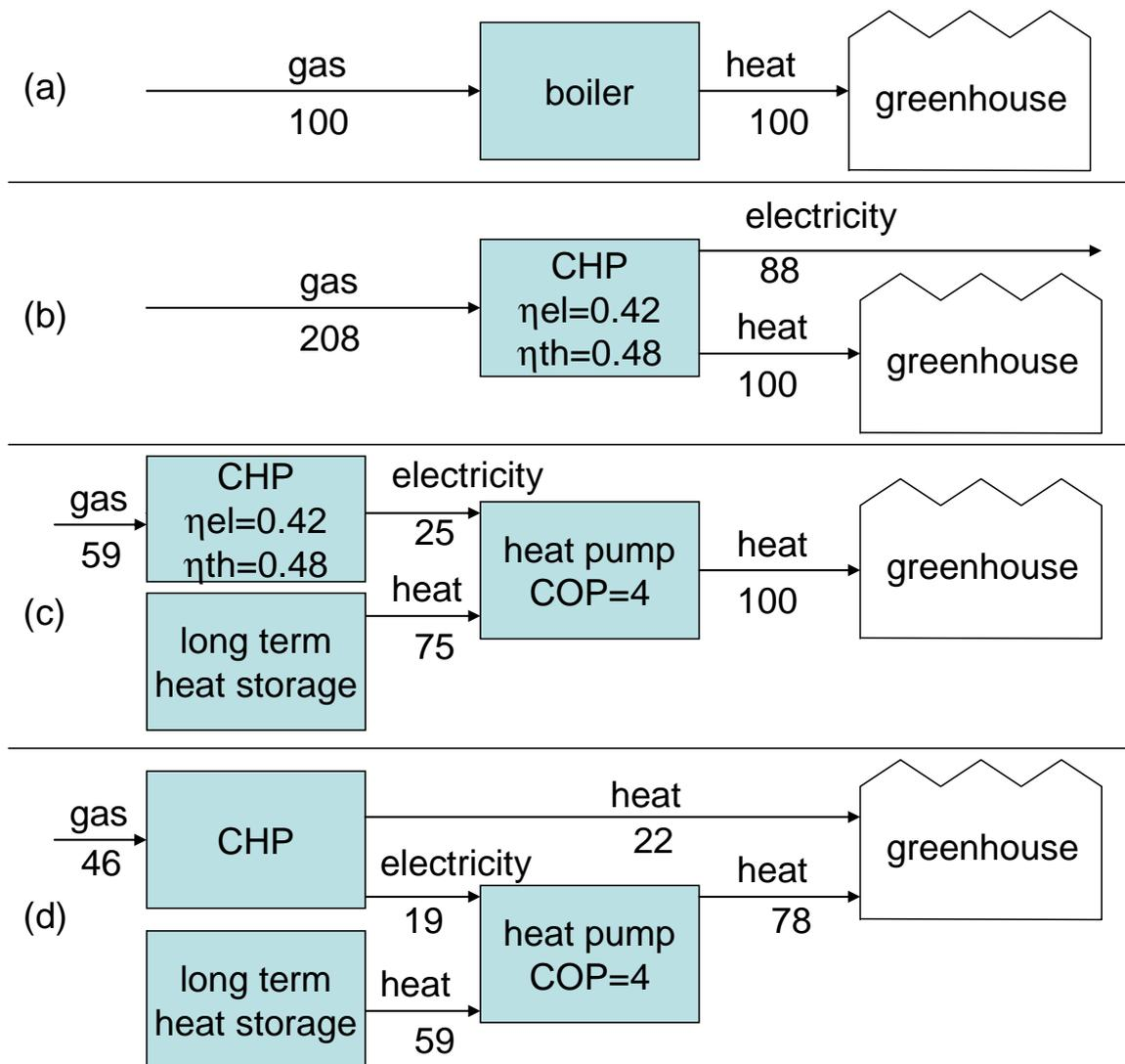
Fig. 7. Simple static calculation of the energy consumption by the energy supply systems at greenhouse heat loss of 100 units, assuming boiler efficiency of 100%, CHP electric and thermal efficiency of 42 and 48% respectively and heat pump COP of 4.
