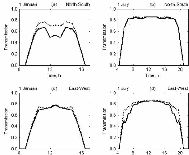
Fig. 3b. The transmitted global radiation of a zigzag covering compared with a standard Venlo glass covering. — Glass covering ..... ZigZag covering
