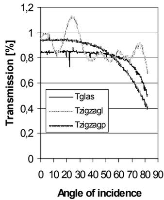
Fig. 3a. Transmission as function of the angle of incidence for incident angles perpendicular (zigzagl) and parallel on the zigzag structure (zigzagp).
