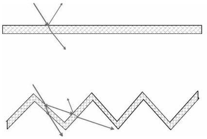
Fig. 1a. The principle of the transmittance and reflection of light beams hitting a flat sheet (above) and a zigzag-sheet (below).
