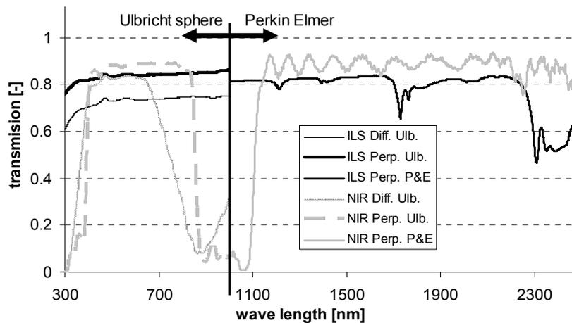
Fig. 1. Diffuse (Diff.) and perpendicular (Perp.) transmission of the ILS ultra (ILS) and 3M NIR (NIR) screen measured in the range of 300–1000 nm with an Ulbricht integrating sphere (Ulbr.) and above 1000 nm with a Perkin and Elmer (P&E).
