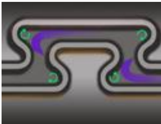
Turbulent flow path with flushing diaphragm Roberts Irrigation.
